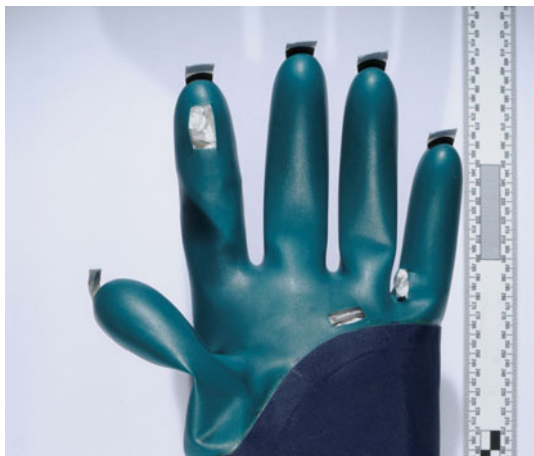
Fig. 1 Typical ACES glove showing samples cut from the index finger, pinky/ring finger crotch, and palm for the neoprene upper area. The lower (darker) glove area below the palm is made of Gore-Tex fabric
